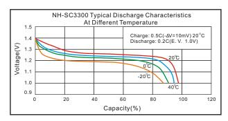
Note: \*Typical values relative to cells stored for less than 3 months or less at 30  $^\circ$ C max.
